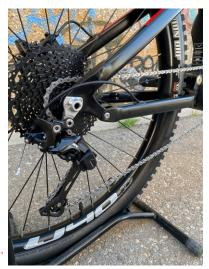
be done at a higher cadence, using larger sprockets, lowering the power delivery of the engine, thus saving battery and wear on components will be less. Shimano recently presented its DEORE XT component range, a specific range for e-bikes, thereby preventing permature wear on the e-bike transmissions.
